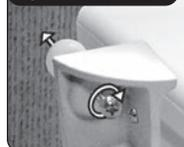
2. Insert the transceiver into the opening.
