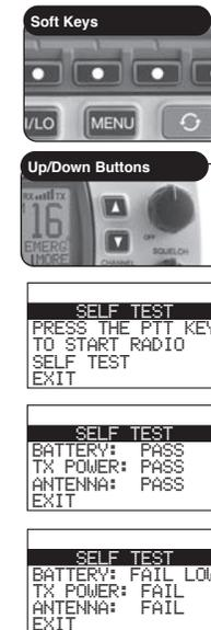
1. Enter the Settings menu and scroll to **SELF TEST** with the **Up/Down** soft keys or the **Up/Down channel** buttons.
